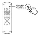
Pressing OPEN/CLOSE opens the tray if it is closed, and closes it if it is open. When the tray is opened during playback, it may take a few seconds before the disc is "unloaded" and the tray opens.
